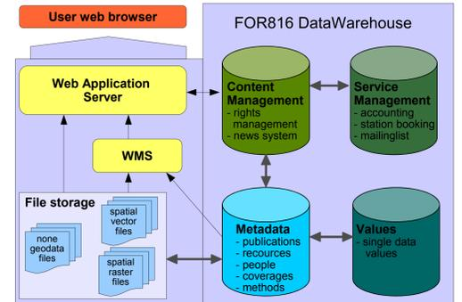
Fig. 4: Schematic system architecture of the FOR816dw
